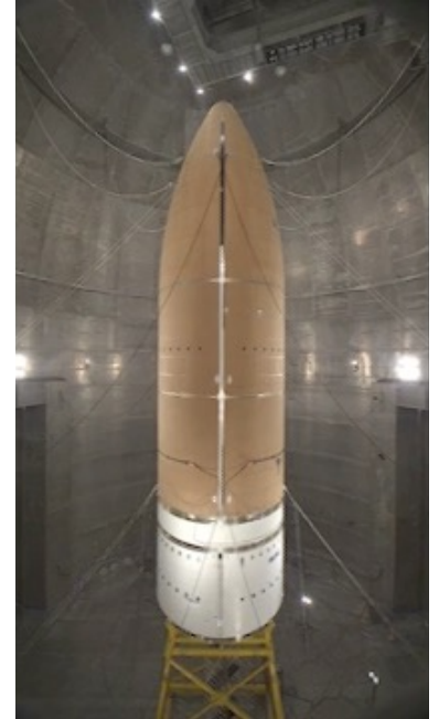
Ariane 5 fairing separation test
